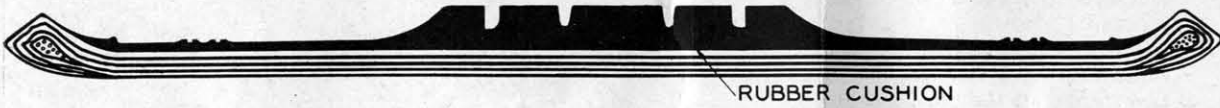
Cross section of full ply Yale tire, showing rubber cushion under tread which permits tread to flex and helps absorb blows. Tensile strength is as much as floating ply tire, while tread strength is from 8 to 10 times greater.
