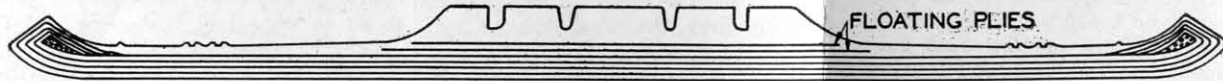
Cross section of tire with floating plies showing why extra plies add no tensile strength to the carcass. They add only weight and stiffness under the tread. Shoulder strength is not helped.
